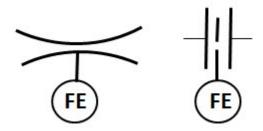
To represent a general flow measuring device in P&ID, flow elements are used.
