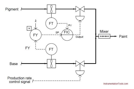
With identical flow range <u>calibrations</u> in both flow transmitters, this multiplying constant k directly determines the pigment-to-base ratio (i.e. the ratio will be 1:1 when k = 1; the ratio will be 2:1 when k = 2, etc.).
