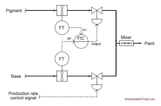
Here, the <u>flow transmitter</u> on the uncontrolled line measures the flow rate of base, sending a flow rate signal to the pigment flow controller which acts to match flow rates. If the calibrations of each flow transmitter are precisely equal to one another, the ratio of pigment to base will be 1:1 (equal).
