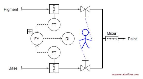
One alteration we could make to this mixing system is to link the two manual control valve handles together in such a way that the ratio of base to pigment was mechanically established.
