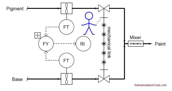
Adjusting the pigment-to-base ratio is now a matter of adjusting the linkage ratio, a task most likely performed by a mechanic or someone else skilled in the alignment of mechanical linkages. The convenience of total flow adjustment gained by the link comes at the price of inconvenient ratio adjustment.
